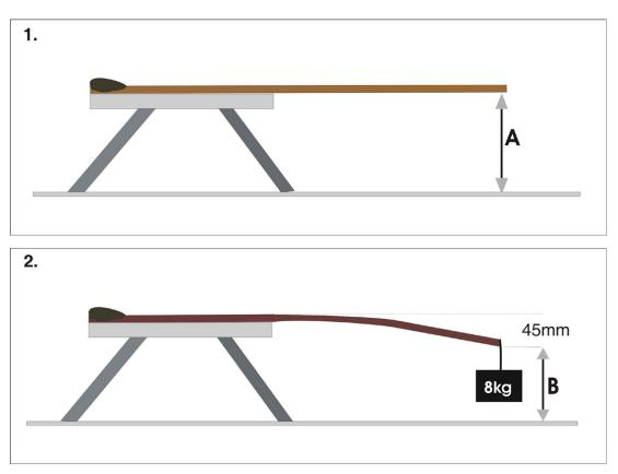
Measure from black band to the floor, and then hang an 8 kg weight on the end. Measure to the floor again, the difference between the 1<sup>st</sup> and 2<sup>nd</sup> measurement is the bend. The gaff should be as stiff as possible sideways.
