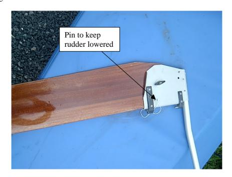
Make sure the tiller is a tight fit in the rudder head. I use a 107cm carbon fibre extension as I like the more positive feel and larger diameter. I had real problems with my aluminium tiller as it kept sliding out of my hand because only the very end had any grip. 107cm is about the maximum you can get away with without giving your crew a black eye and it is just long enough to allow them to steer if necessary.
