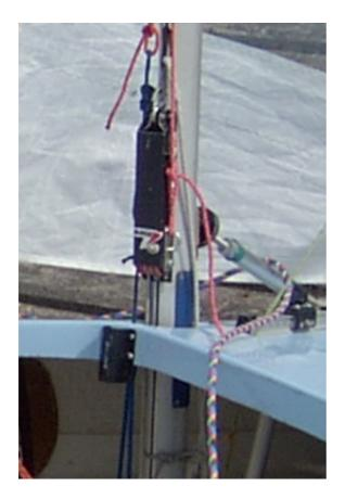
I keep the halyard tidy by hanging it on a plastic hook held on the side of the lower mast with elastic.
