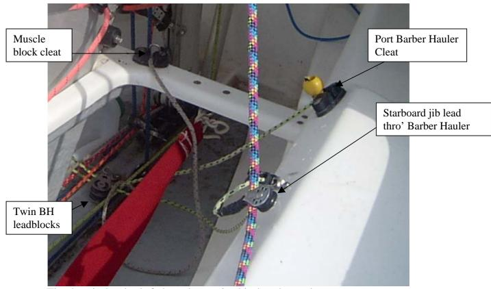
The sheet is then lead aft through a turning block and cam cleat.
