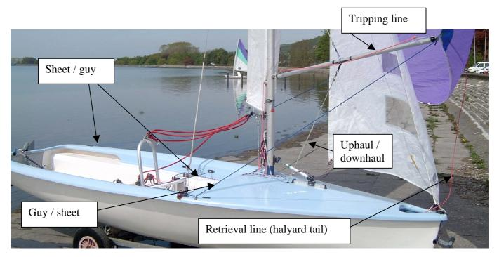
The halyard is a continuous loop from the head of the sail, down the mast and along the port side to a cleat. Then across to the starboard side, under the side deck and out of the spinnaker chute to be attached to the retrieval point on the sail. I have a flexible piece of plastic trim with a wire hook taped to it to make rethreading the halyard easier.
