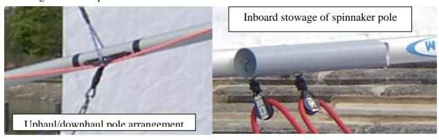
The pole is threaded through a loop in the downhaul/uphaul and the release line tied outside. Thus, in the event of a capsize it is not possible to loose the pole. When stowed one pole end sits in some drainpipe bolted to the side of the boom and the other end is raised by the uphaul to keep it clear.
