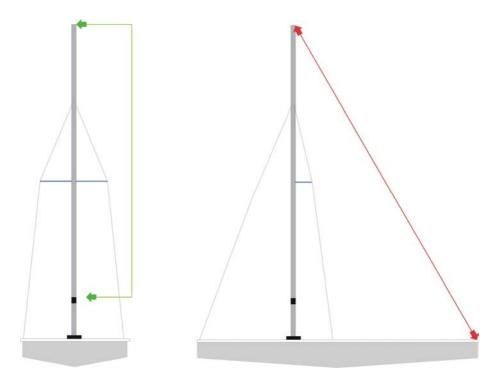
7. With the rake and tension on to the required settings check the pre bend of the mast. To measure this pull your main halyard down to the top of the gooseneck and measure the distance form the aft face of the mast to the halyard. (See diagram 2) This will normally be at spreader height. Adjust until the required spreader deflection is found.
