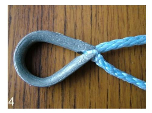
Tighten the eye around the eyelet, or adjust the size of the eye to your requirements.
