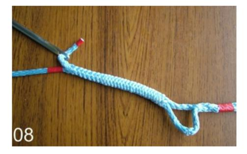
Remove the working end from the needle, and *do not let it disappear inside the braid*. Carefully pull through the braid to remove the loop visible in the lower right of the picture, *but do not smooth out the expanded braid*. As before ignore the misleading piece of tape at the left of the picture.
