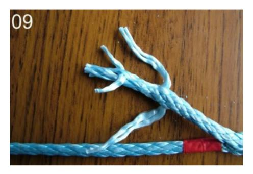
Remove the tape from the working end. Now taper the working end over a distance of a couple of inches, (5cm) by pulling out strands at differing lengths,
