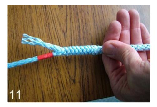
Now ease the braid smooth over the working end, which should disappear into the inside of the tube. Again, ignore the misleading piece of tape.
