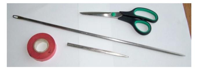
All the tools you need are shown in the picture above. Working from the top we have a *sharp* pair of scissors or you can use a *sharp* knife (it's surprisingly tough to cut), a large darning needle (this was the prototype, and we now use a shorter one), a "fid" – a pointy tubular tool for threading one rope through another, and some ordinary electrician's tape.
