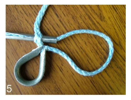
You should now insert the fid as in picture 4 of the long splice, i.e. skip two holes and enter the third, and with the fid at approximately 45 degrees to the standing part, exit at the fourth hole along. You end up with this picture 5 matching the state of play in picture 5 of the long splice.
