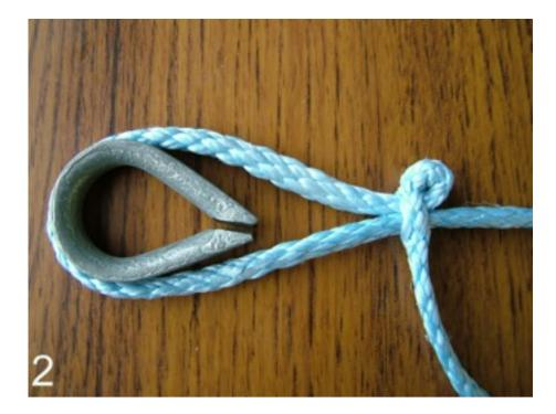
Pull the fid, and the folded bit of the standing part through the hole in the working end. It looks a little odd, but if you pull through, you will create an eye, into which you may or may not decide to put an eyelet, depending on the application.
