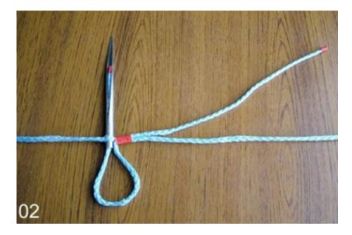
To use the fid, always open up the rope by compressing it gently along its axis, and insert the fid between the strands, adjacent to the tape, and *not* through the strands. Admittedly, this is the fiddliest thing you have to do, but it makes a much better job from a neatness and strength point of view. If you have done it properly, the fid requires very little force.
