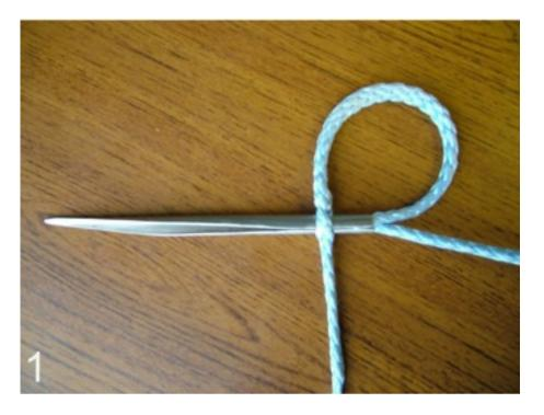
The eye splice is started in a different way to the long splice, but the finishing off is identical.
