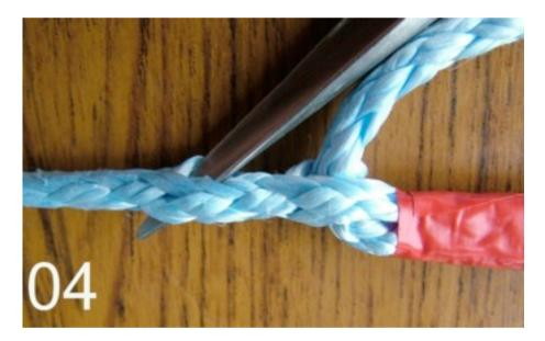
The next step is a fiddly one. When you open up the rope by pushing along its axis you can see little holes where the strands open up. Skip two holes, from the exit point of the first tuck, and push the fid into the third hole at an angle of about 45 degrees, as in the picture. This means that it should come out at the fourth hole on the under side. That's the fiddly bit
