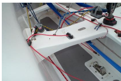
Top Left - Multi-purchase kicker Top Right - The kicker control lines are joined and pass through a hole in the centreboard case. This helps keep the boat tidy. Above - Kicker control line leads
