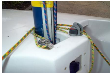
Above - Simple mast ram arrangement is all that is needed, but make sure the block and cleat are man enough for the job.
