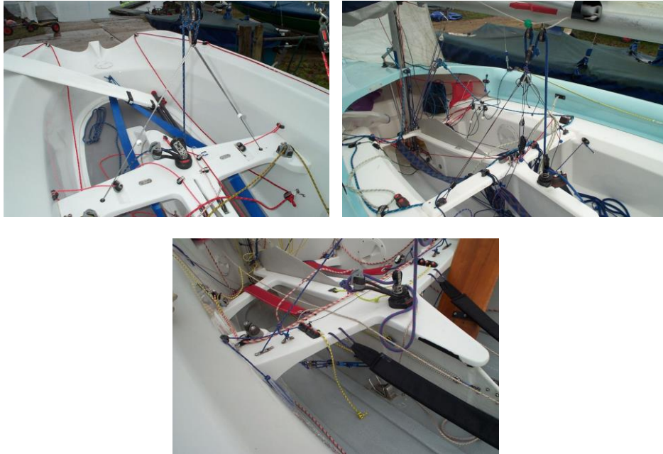
Top Left - Lark 2462 now sports a very clever Herzog adjustable mainsheet bridle first seen on Richard Dowsett's Lark 2331. Top right - Clever but complicated bridle adjustment on Lark 2365 - but it only adjusts the height. Above - Nigel Hufton's Lark 2470 sports a very clever self-tacking mainsheet bridle - nice!
