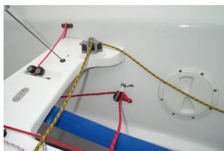
Top left -Continuous barber hauler arrangement on 2462, with single adjustment control line on centreboard case. Top right - Lark 2469 uses very simple jib tracks in place of barber haulers, the tracks could be shorter. Above - Standard positions for Jib and Spinnaker sheets on the new Rondar Lark. Note the fairlead on the jib cleats that help with trimming the jib from unusual positions!
