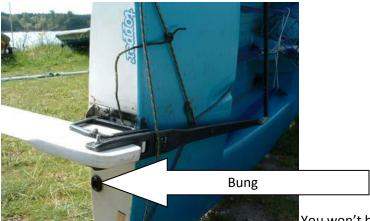
above) until you have enough depth of water ... keep the rudder high until you have enough and then progressively lower the rudder by lifting the tiller and pushing back until the rudder blade is vertical.
