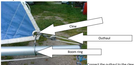
Connect the outhaul to the clew of the sail. Also connect the boom ring to the clew of the sail. The outhaul should be fairly slack unless it is very windy ... in which case pull it tight. Some boats do not have a boom ring –sometimes just a piece of rope that does the same job.
