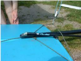
Take the rudder/tiller assembly and from the back of the boat, push it under
