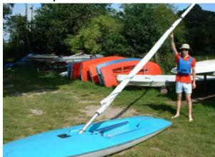
With the mast gate open, insert the mast/sail assembly at this angle. "Walk" the mast upright, as it reaches a vertical position it should drop down into the mast step with a "thud". Shut the mast gate by pulling on the mast gate cord.
