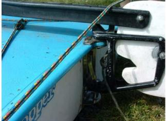
... and then locate the rudder pintle (the pin on top of the rudder)
