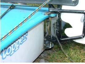
... like this. Topper rudders sink (!) so be sure to tie the rudder
