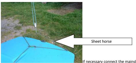
If necessary connect the mainsheet to the sheet horse and make sure that you tie a figure of eight knot in the end or tie the mainsheet to the toe strap.
