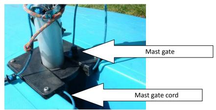
Here's the mast assembly correctly located and the mast gate shut. Check that the fixing for the kicking strap on the mast is facing the back of the boat. Drop the plastic peg in lightly – if you push it in too far, it will be difficult to remove. Now unwrap the sail. If it is very windy, consider leaving part of the sail wrapped around the mast (reefed) to reduce power.
