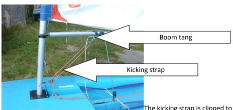
The kicking strap is clipped to the tang on the boom. It is there to stop the boom riding up so ensure that it is tightened by pulling the rope tightly into the cleat on the mast. If it is very windy, do this up very tight once you are on the water.
